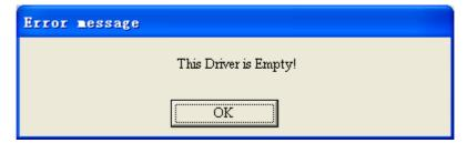
3) When there is a communication failure between the computer and the instrument, the following message will be displayed. Confirm the communication cable and baud rate.
